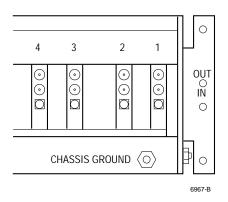
Figure 13. Chassis Ground Terminal
